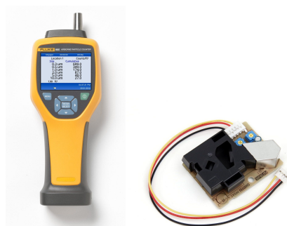
Picture 5. PM can be measured in the air by concentration (mass, for example) or size using particle counters.
